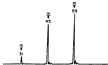
Figure 5. Product ion mass spectrum in the reaction of \text{CH}_3^+ ions with (\text{CH}_3)_2\text{SiH}_2 .
